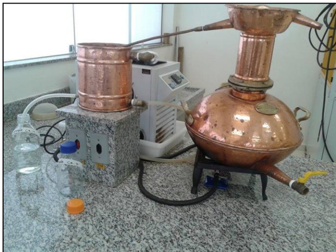
Figure 1. Fifteen-liter still used for the distillation of the fermented must.
